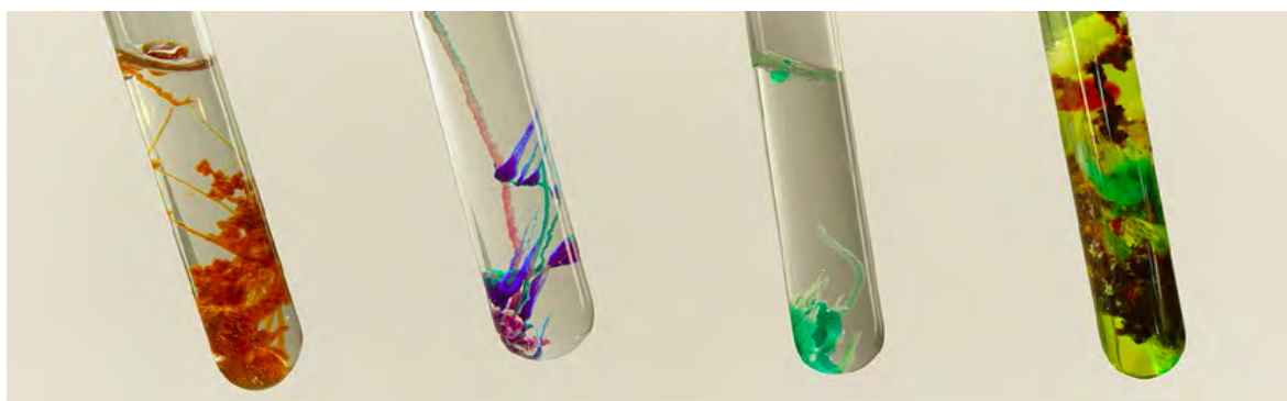
Figure 1: Samples of the "Chemical garden". Each colour is caused by a different metal salt added to the water glass (from TEMI project, 2015, p. 26)
