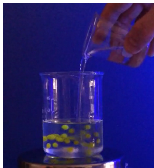
Figure 6: “Turning off” the fluorescence in riboflavin-filled bubbles by adding sodium dithionite solution
