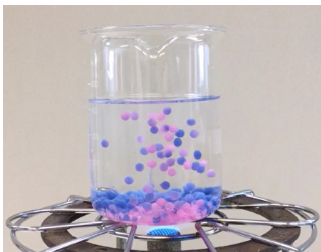
Figure 4: Thermal convection by bubbles filled with thermo ink
