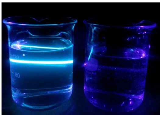
Figure 4: A blue laser light, thrown from the right, passes first through water and then through tonic water whose light blue fluorescence is clearly showed (left). A cube of Plexiglas fluoresces in green when a blue light passes through it.
